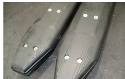
Forks surface with special anti-wear-coating
