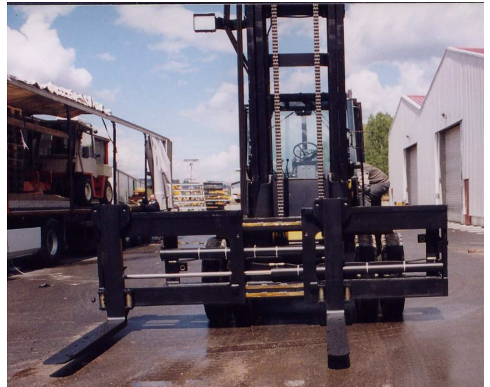
Sideshifter/forkpositioner with adjustable frame width
