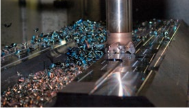
2 fraiseuses 3 axes CN 2200x1000 mm - 1200x450 mm 24 outils
